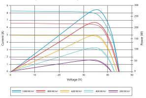
Exellent performance under weak light conditions: at an irradiation intensity of 200 W/m² (AM 1.5, 25 °C), 95.5% or higher of the STC efficiency (1000 W/m²) is achieved
